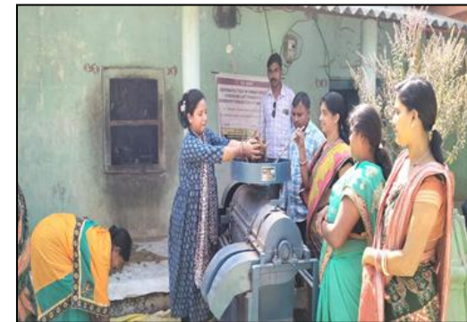
Demonstration of Power operated Finger millet thresher for drudgery reduction of Farmwomen
