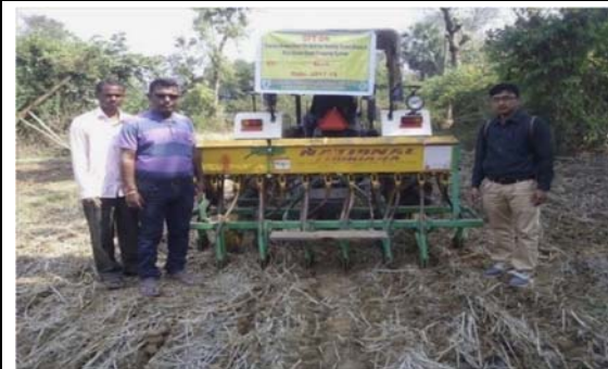
Demonstration of tractor drawn seed cum fertiliser drill for sowing of finger millet
