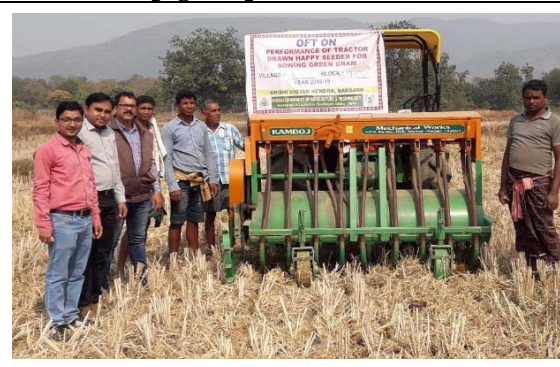
Assessment on Performance of Tractor drawn Happy Seeder for Sowing Green Gram
