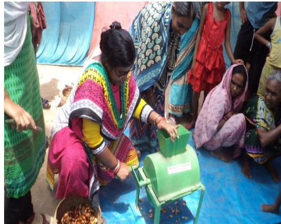
Demonstration of Mahua seed decorticator for drudgery reduction
