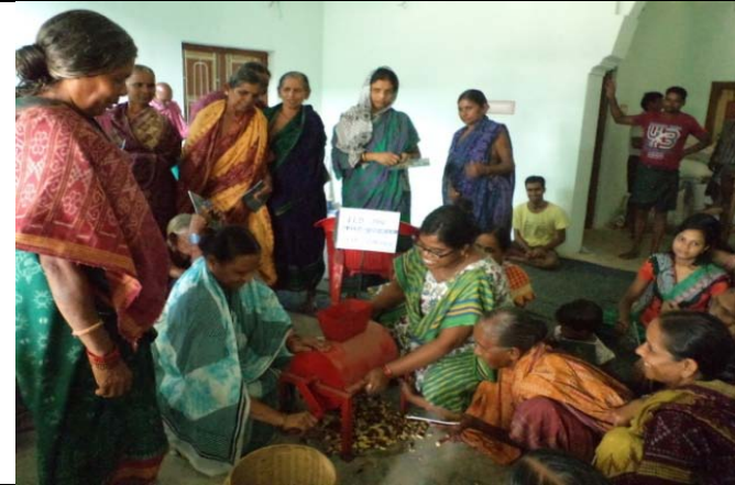
Decortications of mahua seeds done by mahua seed decorticator having weight 14-15 kg made up of mild steel and wooden bar
