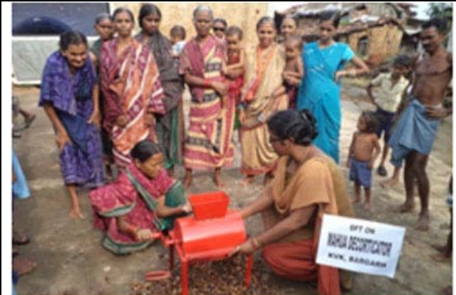
Mahua seed decorticator for drudgery reduction
